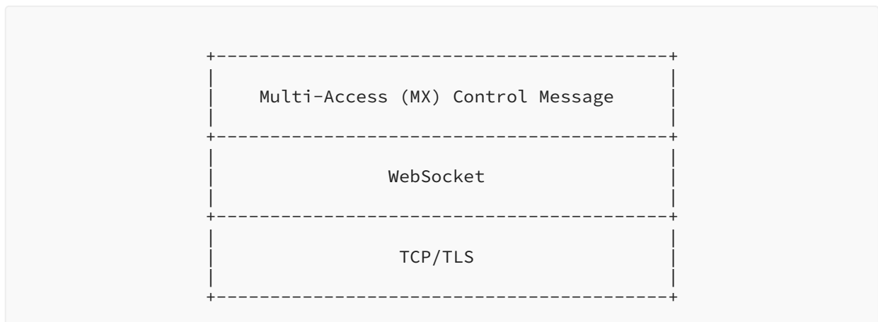
Figure 2: TCP-Based MAMS Control-Plane Protocol Stack
